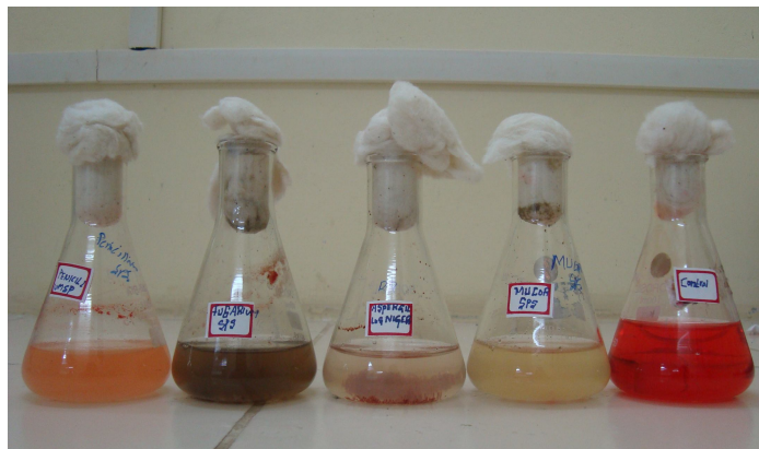
Figure.2 Remazol Red the maximum decolorization was given by the fungi Aspergillus niger (95.9%)
